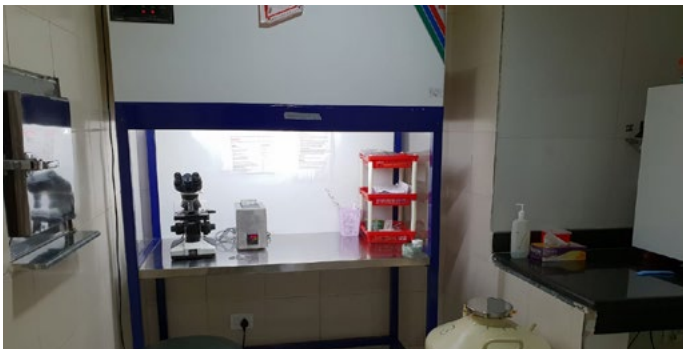
Andrology Lab – Lamina flow hood , connecting air tight window with Semen collection room, Compound microscope, heating block for test-tubes, Cryostorage for sperm samples
