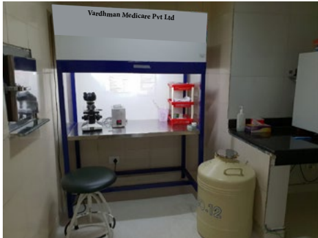
Andrology Lab – Laminar flow hood , connecting air tight window with Semen collection room , Compound microscope , heating block for testtubes ,Cryostorage for sperm samples
